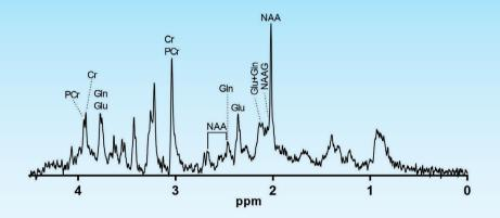
Figure 1: Representative spectrum (upper) from 18 mm<sup>3</sup> voxel covering dorsal striatum (right) based on a STEAM Sequence (TE: 4, TR: 4000 Averages 400) on the Bruker 9.4T microMR. Courtesy of Mikael Palner, NRU.
