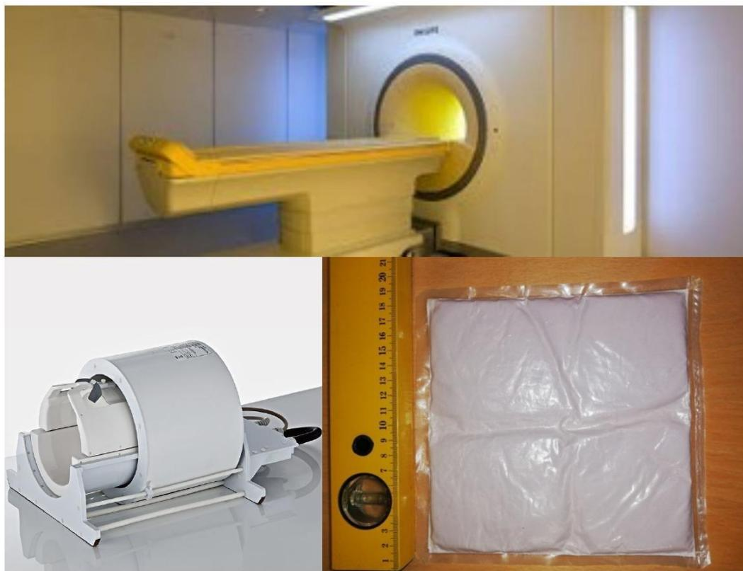
**Figure 2.10.:** *Top:* The Philips Achieva 7T MR scanner at Centre for Functional and Diagnostic Imaging and research, Hvidovre Hospital, Copenhagen, Denmark. *Bottom left:* The head coil (2Tx/32Rx) used for the regular single-transmit setup. This coil is also used in the only FDA and CE approve 7T MR system worldwide. *Bottom right:* One of two dielectric pads, measuring 19x19 cm, that we use in the 7T MRI scans in article 2.
