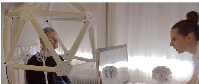
Figure 10: HD-EEG experimental setup. Test person is wearing the 256 channels EEG cap on the head while sitting in the “cage” with the 11 cameras to record the position of the EEG electrodes. To the right Mette Thrane Foged.
