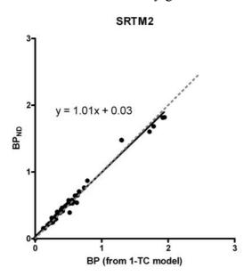
**Figure 5.** Correlation between  $BP_{ND}$ 's calculated from [<sup>11</sup>C]SB207145 PET data using a 1-TC model and SRTM2.  $R^2 = 0.98$ .
