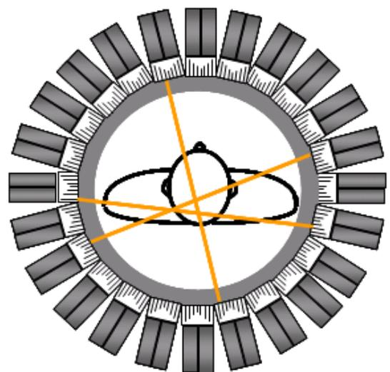
**Figure 3** Detectors register the emitting photons from the subject in the PET scanner (Drawing kindly provided by Brian Lopresti, PhD)
